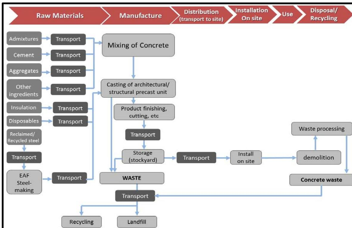
Different “unit processes” associated with the Cradle-to-Grave service life of architectural/ structural precast units.
